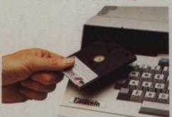
BUILT-IN DISC DRIVE 500K 3" compact floppy disc drive. Potential for massive extra storage with a second 500K disc drive internally.
